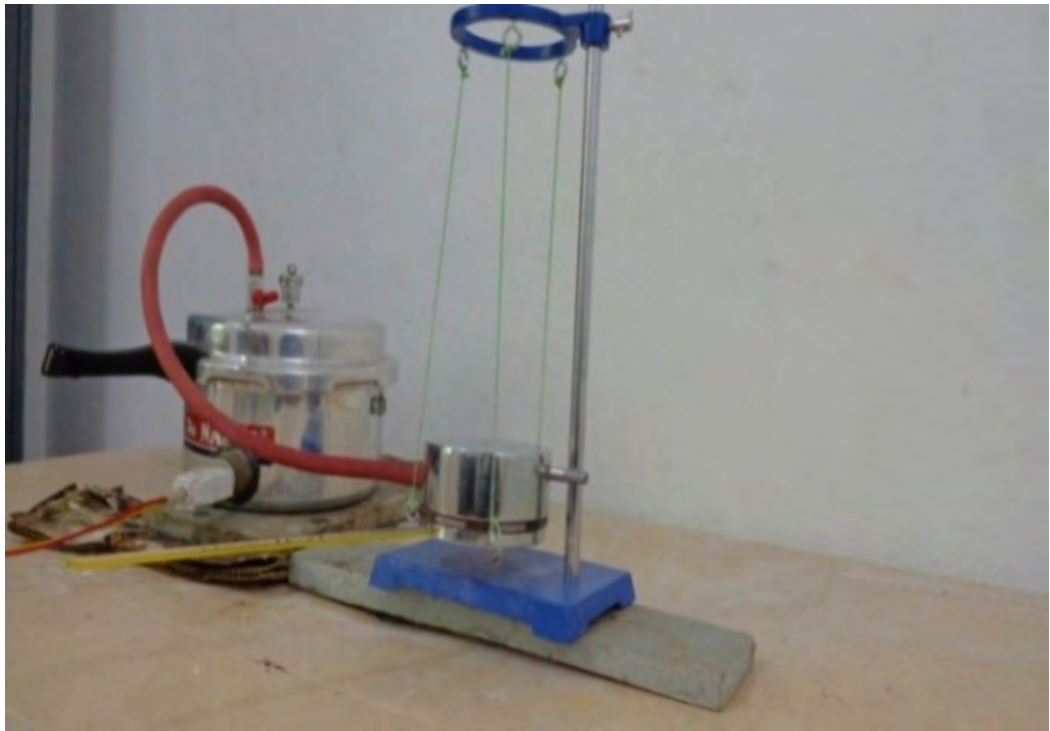
Figure 4: Lees's Disc apparatus[10]
